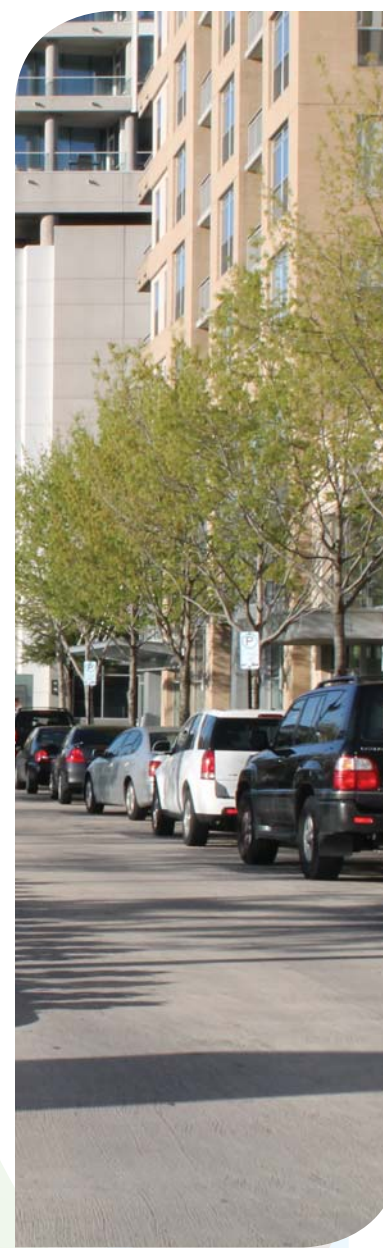
On-street parking creates side friction and reduces vehicle speeds.
